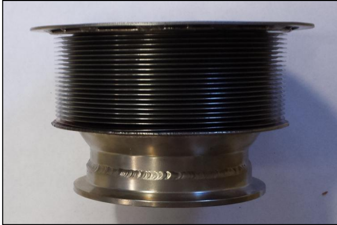
Figure 4: Example of mechanical bellows used as secondary source
